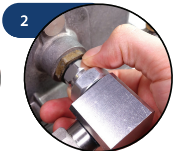
2 Tighten coupling nut to secure in final position
